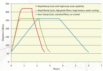
A robust filter design and unique filter retention system minimizes stress from thermal expansion and contraction to maintain ISO Class 5 (Class 100) conditions throughout the cycle even at accelerated heating and cooling rates. These high temperature HEPA filters require no burn-in at installation. ISO Class 5 (<100 0.5 micron particles per cubic foot) performance is guaranteed by Despatch and can be certified as part of the final acceptance test.
