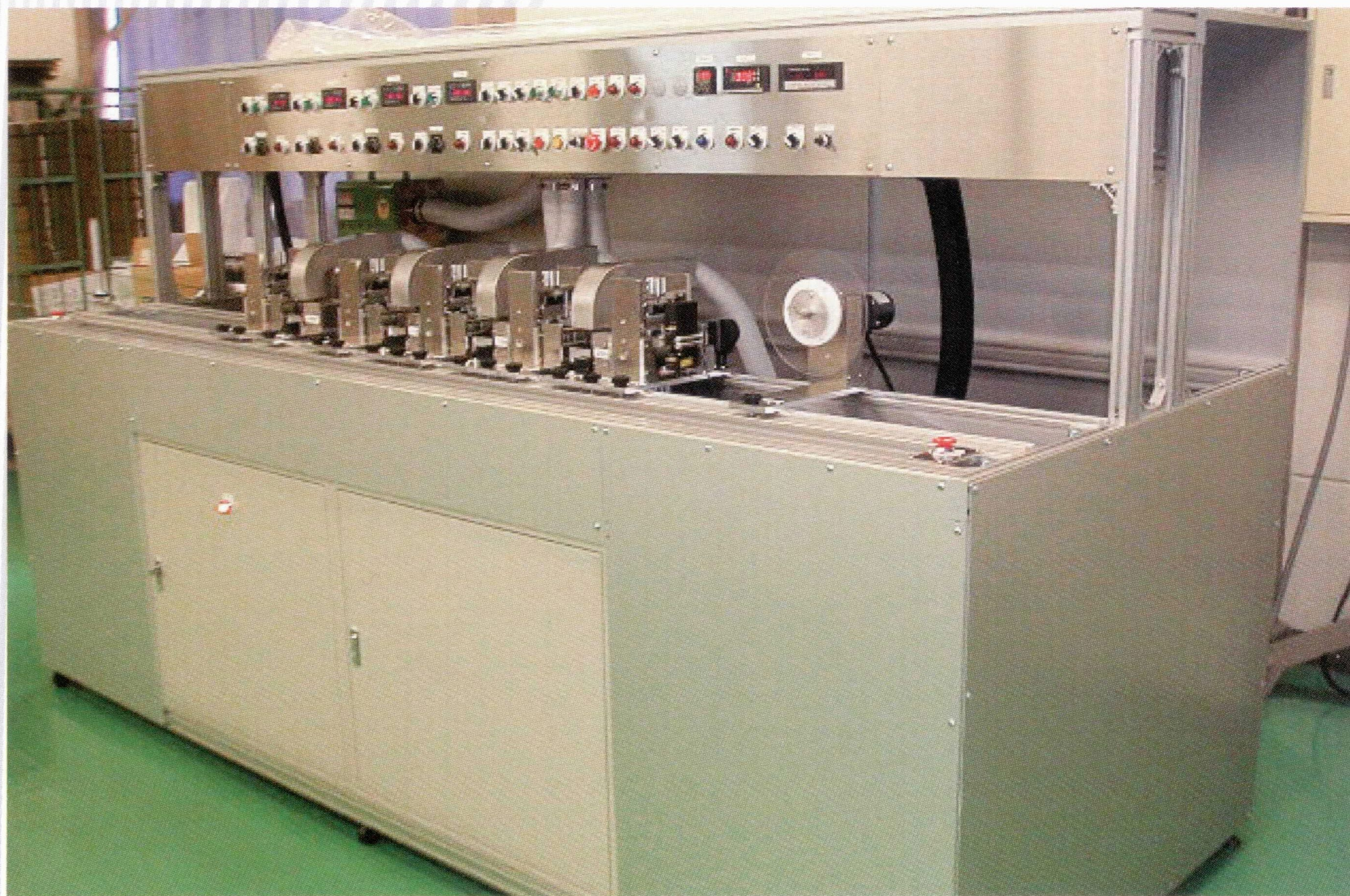
一錘式開織装置 Single-tow Spreading Machine
